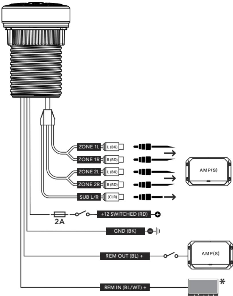
\* Optional connection to a source unit's remote turn-on output (+12V). If used, the MBT-CRXv3 power button will no longer operate.
