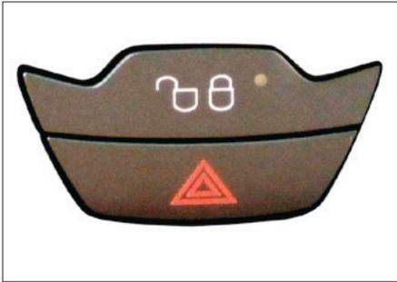
15. A spare OEM hazard light switch by Ford is required.
