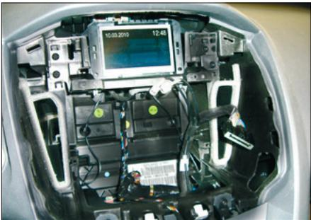
9. OEM dash board with removed head unit
