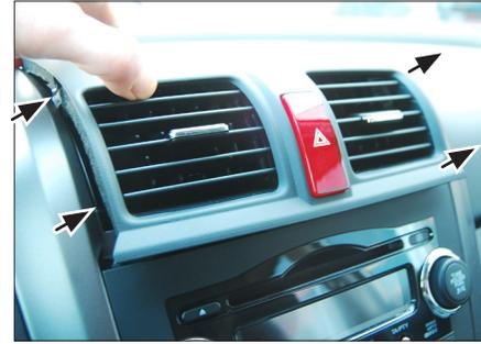
4. Remove the air vent unit
