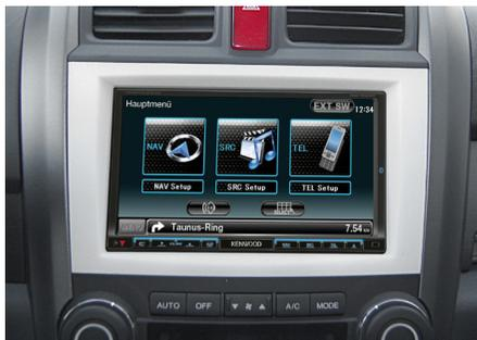
8. Connect all required circuit points and push the double DIN head unit in the metal frame until it snaps in.
