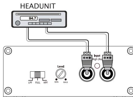
The high-level input(s) should only be used if the RCA output are not present, connect the speaker outputs from the receiver to the high-level input connector of the amplifier. Be sure to observe polarity to avoid audio phase problems.
