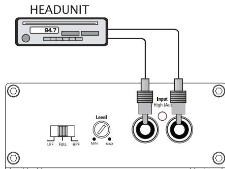
Low-level (RCA) input wiring is preferred for best audio performance. Always use a high-quality cable.
