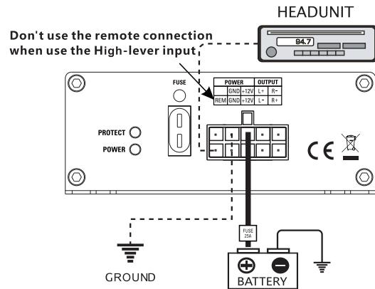
Connect an empty fuse holder within 18" (45cm) of the car battery and run 8 gauges cable from this fuse to the amplifier location. Then connect the fuse holder to the battery +12 Volts.
