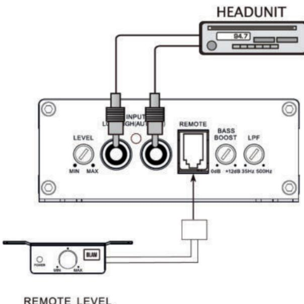
Low-level (RCA) input wiring is preferred for best audio performance. Most trunk or hatchback installations will require a 15-20 feet RCA cable, while pickup trucks and under-seat installations will require a 6-12 feet RCA cable. Always use a high quality cable. Connect to remote turn-on terminal head unit.
