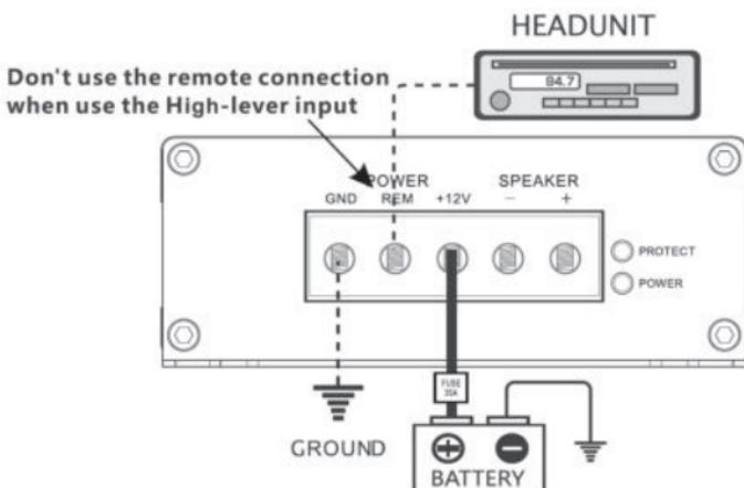
Connect an empty fuse holder within 18" [45 cm] of the car battery, and run 8 gauge (or heavier) cable from this fuse to the amplifier location. Then connect the fuse holder to the "BATT+". Connect the ground terminal to the closest point on the chassis of the vehicle. Keep this ground wire to less than 39" [100 cm] in length. Ensure that the contact surface is free of paint or rust so that the connection between the terminal and the chassis is effective.
