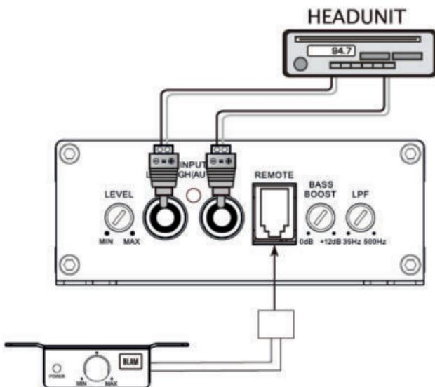
The high level input(s) should only be used if the RCA output are not present, connect the speaker outputs from the receiver to the high level input connector of the amplifier. Be sure to observe polarity to avoid audio phase problems. The AUTO POWER ON is for high level connexions. The subwoofer turns on automatically when there is a signal on the input.
