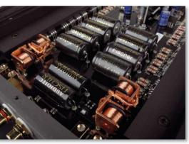
The most elegant solution for a protection circuit: Two separate relays made of solid copper separate the loudspeakers when necessary, naturally process-controlled.
