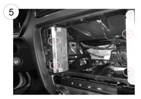
Connect all cables to the Pioneer head unit. Insert the head unit into the dash and check correct operation of the head unit. Secure the head unit into place in the circled positions, using the four small screws supplied.
