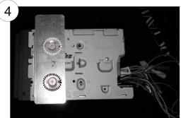
Attach the remaining two brackets to the Pioneer head unit using the screws supplied.
