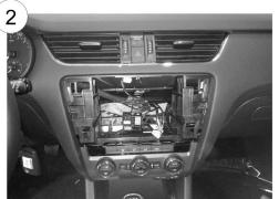
Carefully unclip the original panel with plastic panel removal tools. Remove the OEM head unit by inserting four release keys. Keep the white panel clips holding the facia in place for use later in step 6.
