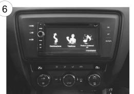
Take the supplied facia plate and attach the white panel clips removed in step 2. Mount the facia over the Pioneer head unit. Installation is now complete.
