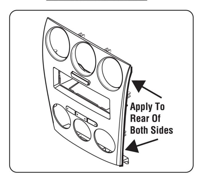
**Note:** Due to differences in factory tolerances you may need to apply the provided felt tape to the edge of the **facia** radio housing to relieve backlight bleed through.
