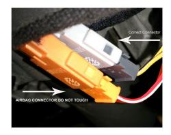
7. Connect the female vehicle specific connector to the male vehicle connector. Test head unit for correct operation.
