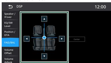
$\blacktriangleleft$  and  $\triangleright$  adjust the left and right volume balance.
