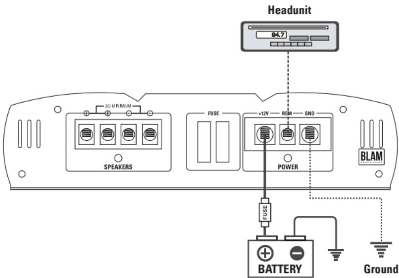
Connect an empty fuse holder within 18" (45 cm) of the car battery, and run 8 gauge (or heavier) cable from this fuse to the amplifier location. Then connect the fuse holder to the "BATT+". Connect the ground terminal to the closest point on the chassis of the vehicle. Keep this ground wire to less than 39" (100 cm) in length. Ensure that the contact surface is free of paint or rust so that the connection between the terminal and the chassis is effective.
