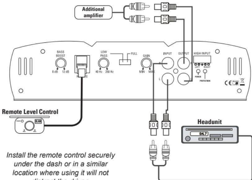
Low-level (RCA) input wiring is preferred for best audio performance. Most trunk or hatchback installations will require a 15-20 feet (4.6 meters) RCA cable, while pickup trucks and under-seat installations will require a 6-12 feet (1.8-3.6 meters) RCA cable. Always use a high quality cable. Connect to remote turn-on terminal head unit.
