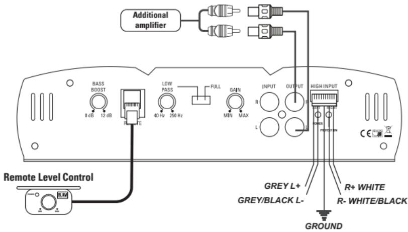
The high level input(s) should only be used if the RCA output are not present, connect the speaker outputs from the receiver to the high level input connector of the amplifier. Be sure to observe polarity to avoid audio phase problems. Connect to remote turn-on terminal head unit.
